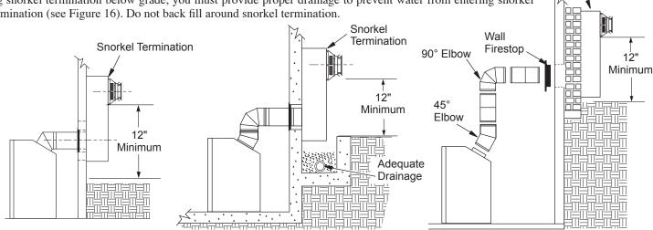
Figure 16 - Snorkel Termination Configurations for Below Ground Installation
